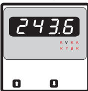
Screen 2 : System Voltage max Value Value displayed after "Hi" flashing on Display
