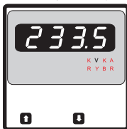
Screen 3 : System Voltage min Value Value displayed after "Lo" flashing on Display
