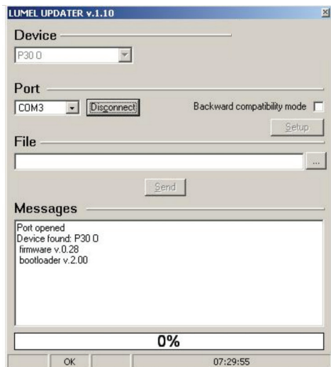
Fig. 27. Screenshot of the software for updating transducer firmware
